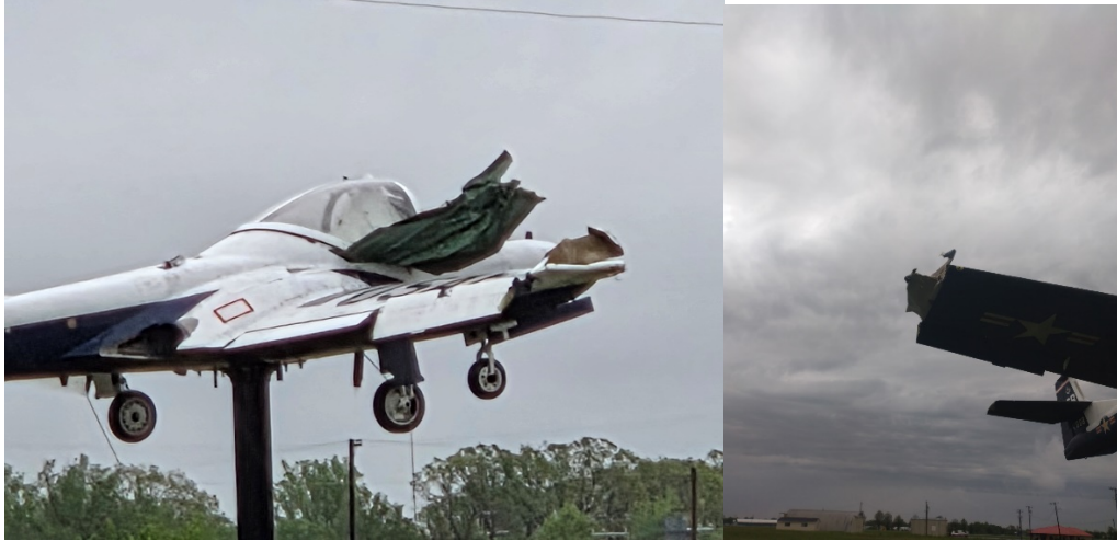
damage to the right wing leading edge, damage to the right-side stabilizing cable
