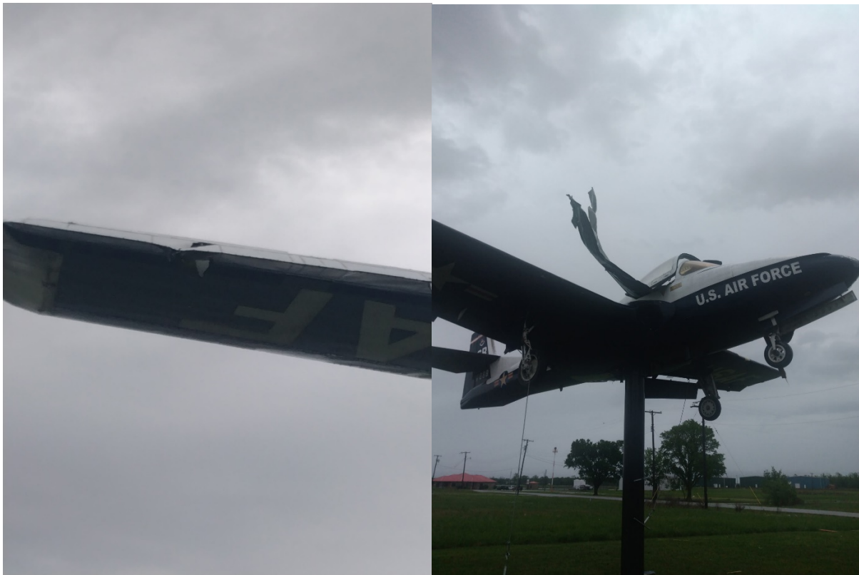
damage to the right wing leading edge, damage to the right-side stabilizing cable
